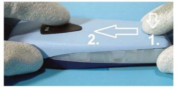
Release the A-Cover from the bottom side of the unit.
