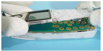
Take away the Display Assembly (UI module) and avoid touching the pads.
