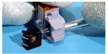
When re-assembling the Microphone remember the right direction. The opening of the Microphone has to point to the opening of the connector housing.
