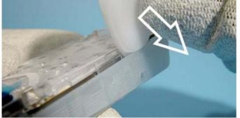
When releasing the side clips of the D-Cover you can use the SRT-6.
