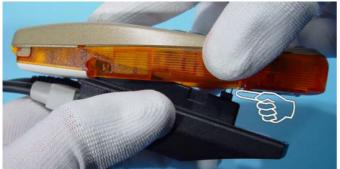
Insert the Flash Adapter FLA-23 like a battery, start at the battery connector site.
