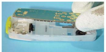
The next step is to take away the Radio Module. Take care not to damage the LED's.
