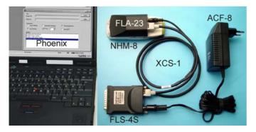
It is very important to follow this insertion and removal procedure, otherwise the contact pins of Flash Adapter will be damaged.
