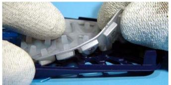
Also, protect the inner part of the window with a foil. The Keymat is loose inside the A-Cover.
