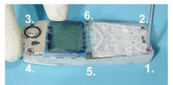
Unscrew the six T6 screws, using the order shown. For assembly, the reverse order and a Torx T6 PLUS with a torque of 28 Ncm has to be used.
